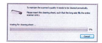
3. Place the cleaning sheet in the scanner. Place the damp side face down.
