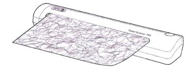
4. The scanner pulls in the cleaning sheet. The scanner will move the cleaning sheet back and forth during cleaning.
